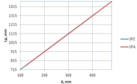
Fig. 2. The variation the primary length with the axis distance
