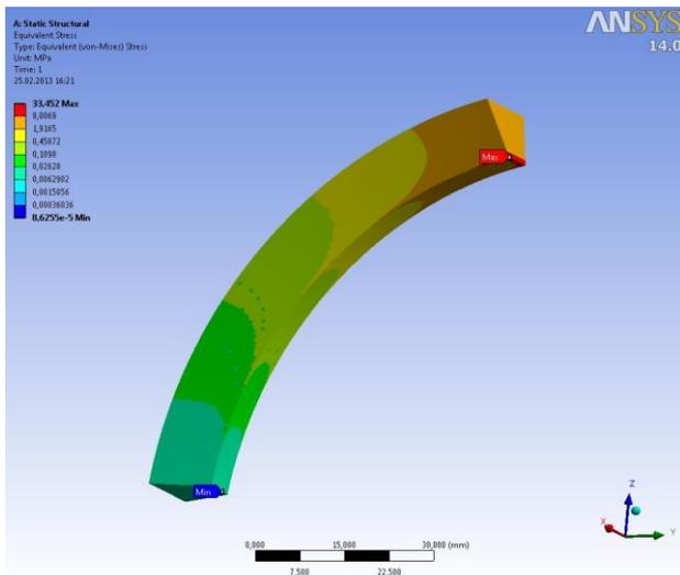
Fig. 9. The distribution of the equivalent stress, for the SPA belt
