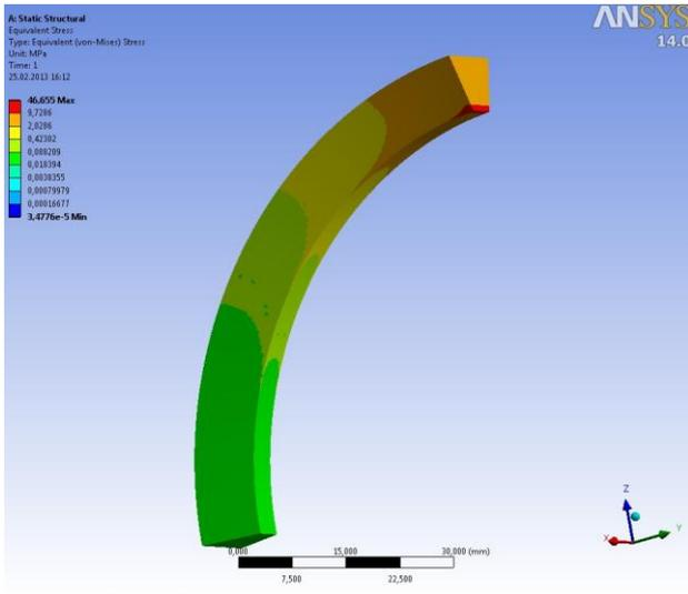
Fig. 8. The distribution of the equivalent stress, for the SPZ belt
